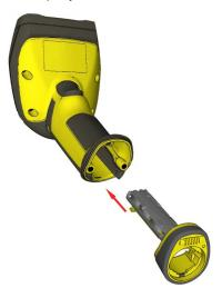
2. With a 2.5 mm Allen wrench, tighten the screws so that the slide-in is firmly locked.
