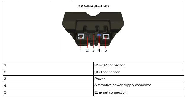
Observe the following electrical requirements when connecting the base station through RS-232:
