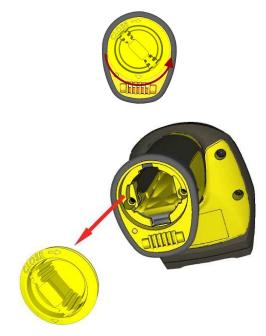
2. Hold the reader in an upright position and the battery slides out of the handle.
