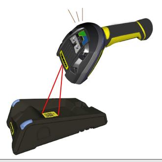
Note: Scanning the Pair code puts the base station and the reader into *force pairing mode*. This means that the reader and the base it is put on get paired regardless of any assignments they both had previously. This force pairing mode is valid for 20 seconds after reading the Pair code.
