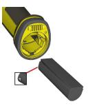
Note: Remove the battery from your DataMan 8072 DL before inserting/removing the communication module.
