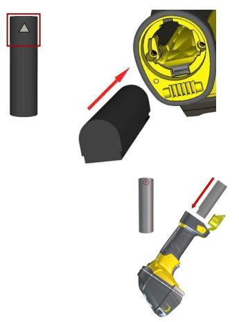
4. Put the end cap back on and twist it. Make sure that the triangle aligns with the circle when the cover is locked.
