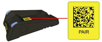
The reader then blinks GREEN/BLUE until it gets paired with the base station (or until the end of the 20 second timeout period). When placing the reader on the base station, the base station drops its pairing with its old reader and pairs with the new reader.
